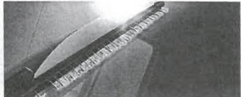
The WET WIPER SYSTEM 1 offers the driver the best possible visibility whilst the blades wash the windscreen.
